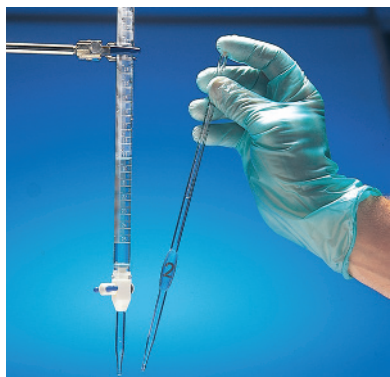
Figure 1.8 Measuring volume. A buret ( left ) delivers an accurately measured variable volume of liquid. A pipet ( right ) delivers a fixed volume (e.g., 25.00 mL) of liquid.
