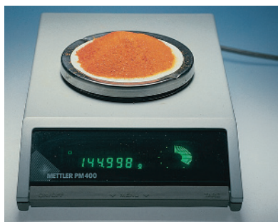
Figure 1.9 Weighing a solid. The solid sample plus the paper on which it rests weighs 144.998 g. The pictured balance is a single-pan analytical balance.
